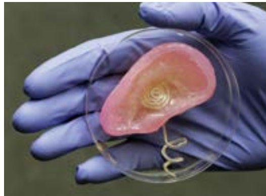
Princeton engineers used 3-D printing to create an ear made up of a coil antenna and cartilage, demonstrating an efficient method of merging electronics with tissue.
